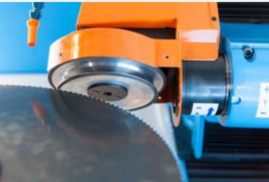
Sharpening the clearance surface and bevelling
