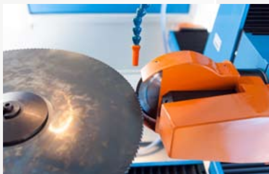
Sharpening of the face and tooth profiling
